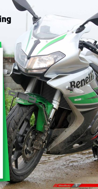
he Benelli Tornado 302R is powered by a 300cc engine that produces 38.26 BHP at 11k RPM, and a maximum torque of 26.56Nm at 10k RPM. The engine is mated to a 6 speed gear box. Crank the engine and my God, the exhaust note sounds so bassy. Rev it up post 8000rpm you can hear a totally different exhaust note from the machine. The engine feels a bit sluggish when it is compared to the TNT300. Small vibrations are felt at around 5000 RPM range.
