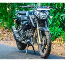
grunt to easily pop a wheelie whenever you want it to, this, on the other hand, is a 200 so you can imagine what all stuff it can do. The engine is a SOHC unit which produces 18 Nm of torque. Combine this with Apache's Racing throttle response (RTR) and you get a bike which can accelerate from 0-60 in just 3.6 seconds. That's impressive for a 200cc motorcycle.
