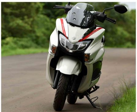
Alongside the center located LED headlamp there are DRLs, Suzuki has introduced LED at both headlight and tail lamp. Coming to the rear section of the scooter, it is nicely designed, although as mentioned earlier as compared to the massive front it looks subdued. The rear blinkers come integrated with the LED taillight coupled with huge grab rail. From side profile also the Burgman looks immense, containing the signature Maxi scooter front paired with Jet-ski type handlebar and extra long seat.
