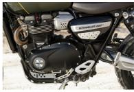
Triumph Scrambler uses the same liquid-cooled T120 engine but churns out 88.7 HP at 7,400 RPM and 119 Nm of torque. In comparison, the T120 in its stock state produces 79 HP at 6.550 RPM and 105 Nm of torque at 3.100 RPM.
