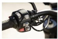
Triumph Scrambler 1200 comes with six riding modes, dual channel cornering ABS, optimised cornering traction control, and a lot more. Five of the six modes are available on the XE version and all of them can be found on the XC variant. The additional mode is "off-road pro" which turns off the ABS and the traction control while simultaneously switching to a different dedicated throttle map.
