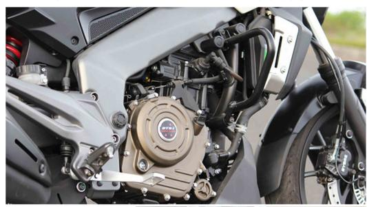
The tuning of this engine is according to the last gen KTM 390 engine, as it produces almost the same torque (35 NM @6500 RPM). The power of the engine is reduced to 35 PS @8000 RPM to ensure that it remains stress-free under long riding conditions. Many people are also
