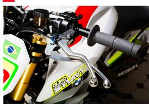
While performing rotating wheelies, quick-slides, or any other stunt which requires the rider to stand on the rear seats, a handbrake lever is used. Its job is to provide the option of braking from the rear wheel, without using the foot lever. In this setup, an additional caliper is installed beside the stock one on the rear disc and an adjustable handbrake lever is connected to it on the handlebar.
