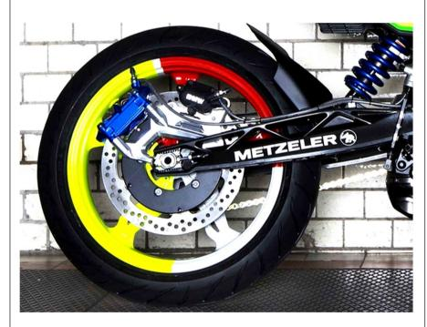
The brakes on a stunt bike need to give a lively feedback and an instantaneous bite from the steel discs. While the steel braided lines take care of the pressure feel and the feedback, a new calliper, preferably a multipiston one, gives you the required bite. The pressure by default is kept quite high in these lines to facilitate stoppies even at the lowest of speeds.
