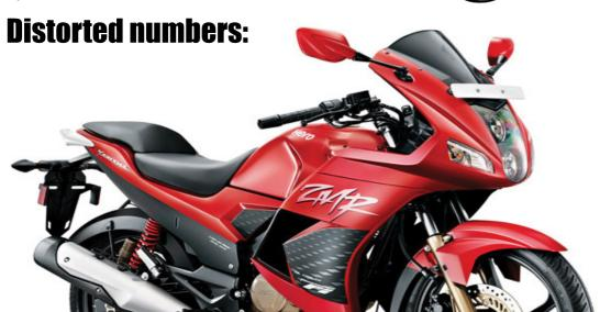
The bike has a ground clearance of just 145 mm but an unusually high seat height of 810 mm. The non-conventional numbers make you feel that you're sitting high up but a lot of time, you end up scraping engine belly. Karizma feels very bulky to ride because of it's abnormally high length (2100), breath (805) and height (1190). With these numbers' it feels like the bike was originally intended to be a cruiser but mid-way along its development the plan was changed.
